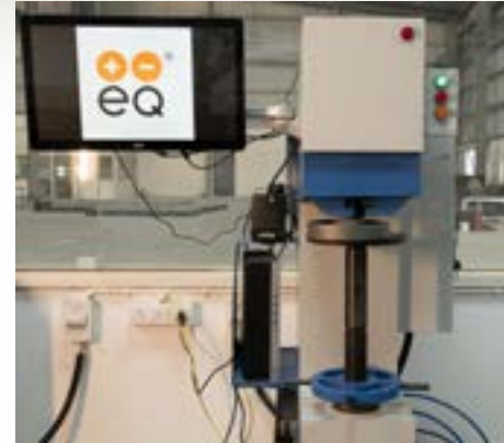
Brinell hardness tester
